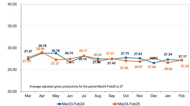
Productivity is determined by averaging the number of containers lifted per hour per crane during the time vessel operations are underway. Vessel operation time is determined by the time the vessel is at berth minus delays.
