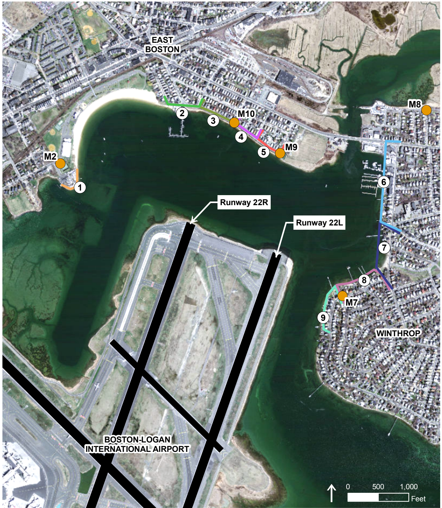
Figure 4-12 Runway 22R Noise Monitoring Locations and Receptors
