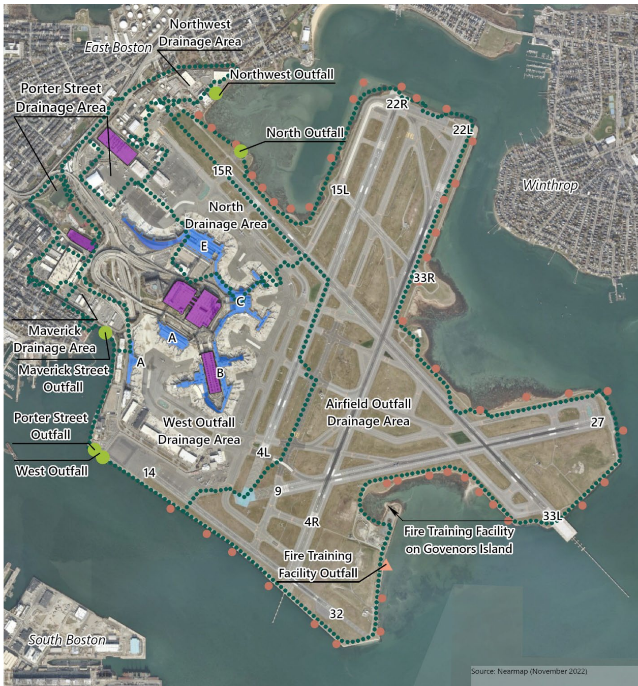
Figure 9-1 Logan Airport Outfalls
