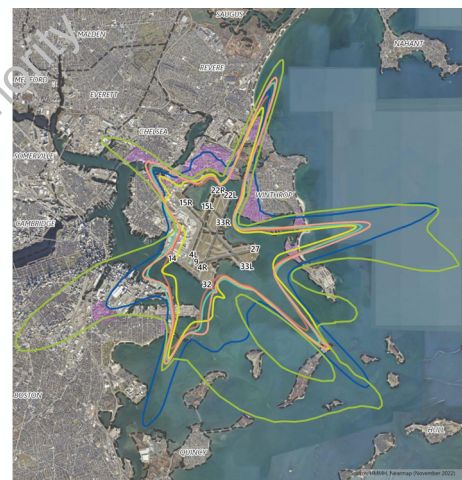
Figure 7-22 Comparison of 1990, 2000, 2010, 2019, 2022, and 53.5 MAP 65 dB Contours 2022 Environmental Status and Planning Report 65 dB Contour by Year/94L 1990 2000 2010 2019 2022 53.5 MAP Residential Sound Insulation Areas Municipal Boundary 0 3,500 7,000 Feet
