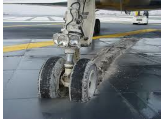
Figure 1-2 Aircraft Gear in Engineered Materials Arresting System (EMAS) (Photo Credit: SKYbrary, 2020)
