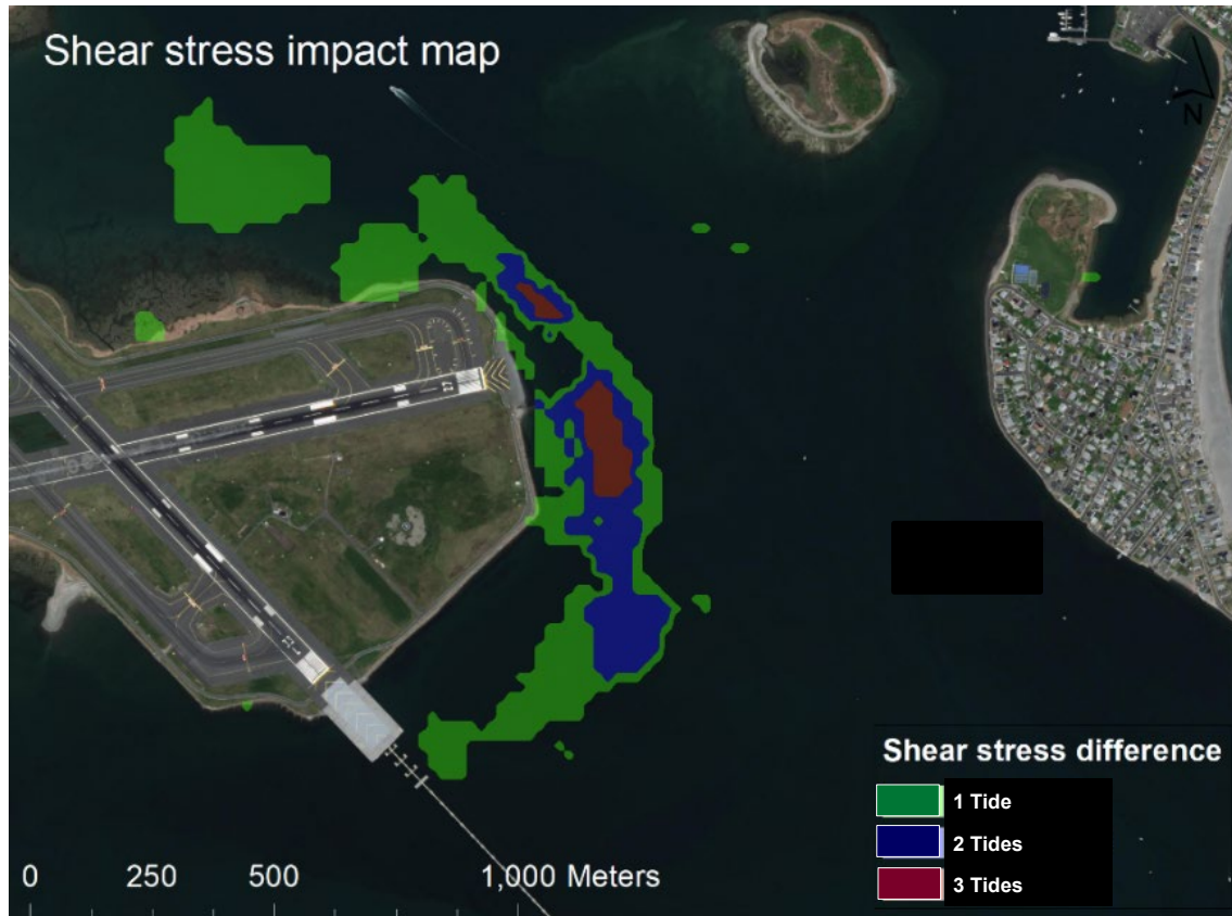
Figure 4-4. Impacted area due to change in shear stress with the combined effect of high, mid, and low tide conditions
