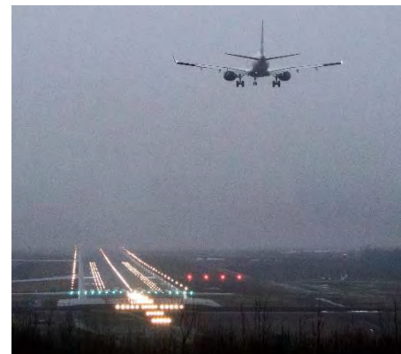
CAT III Instrument Landing System. Source: Massport.
