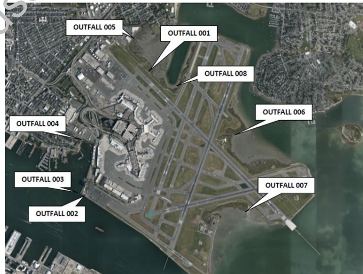
Logan Airport stormwater outfalls
