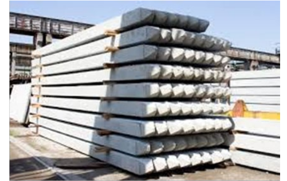
Precast concrete piles
